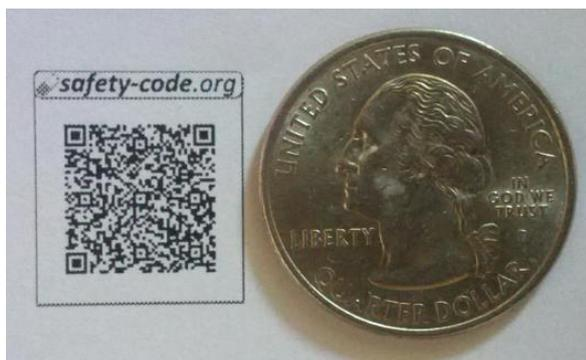
**Figure 3: An example of a printed MSC. The QR code in this example had a side length of 1,15 cm and was readily decoded with the smartphone device used for proof-of-concept testing.**
